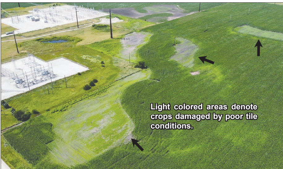
Drainage tile is damaged due to expansion at a utility site in rural Iowa.
